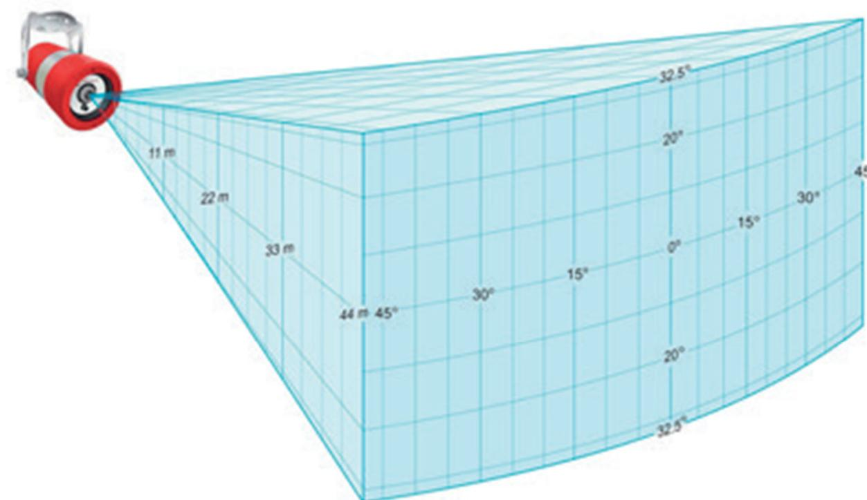
Software analysis of the actual detector coverage may be required to ensure adequate coverage of the hazards. This analysis can also be used to optimise the number of detectors.
