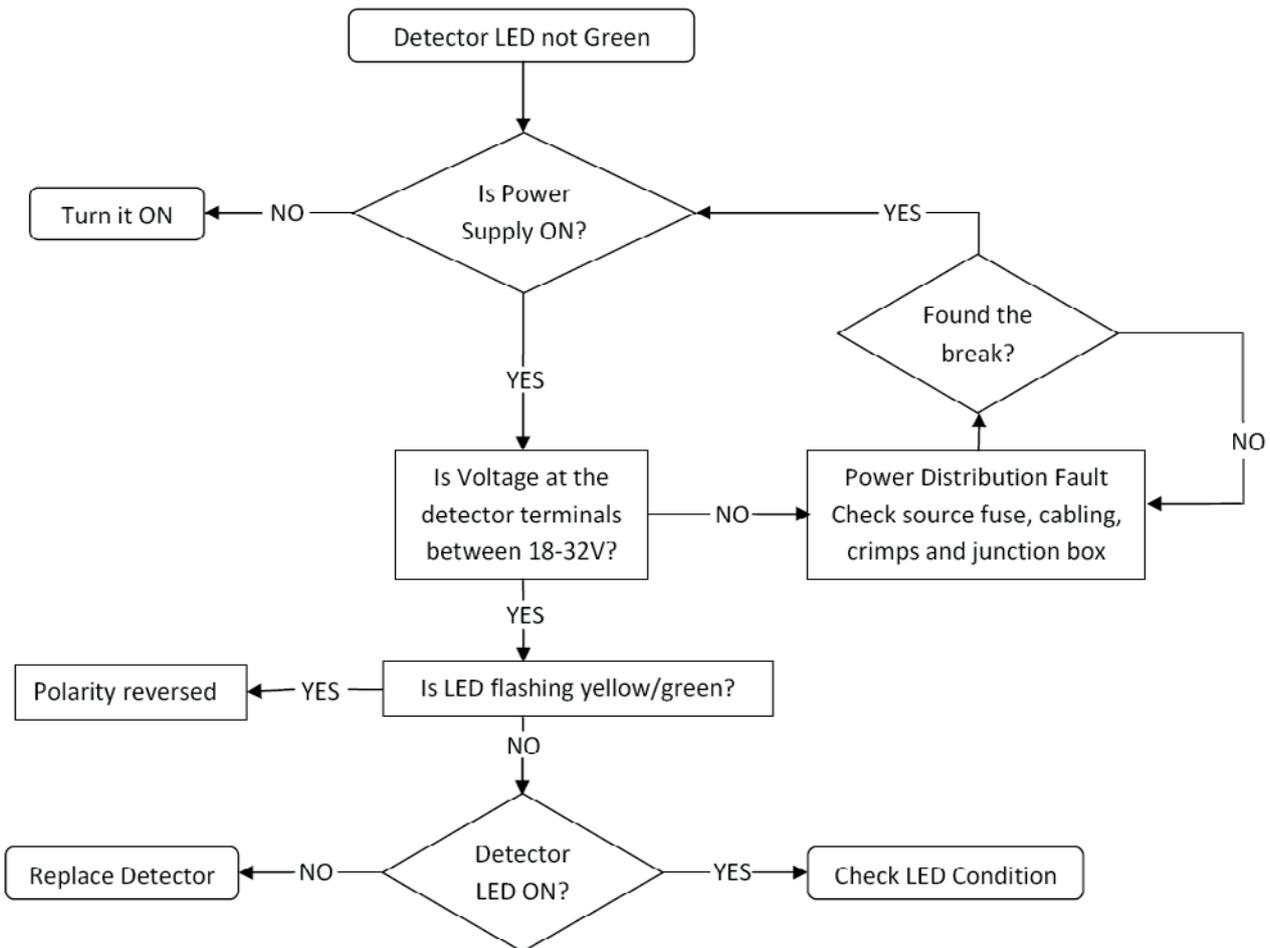
When investigating power supply faults it is important to check that all voltages are within the detectors operating range (18V to 32V) under full load conditions as the voltages measured under no load conditions can be misleading.
