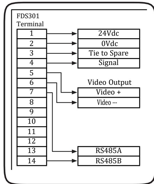
\*Tied to spare terminal at control panel to allow RS485 communication with detector. Both HART and RS485 cannot co-exist in a detector. When the power to the detector is reversed RS485 is enabled in this configuration.
