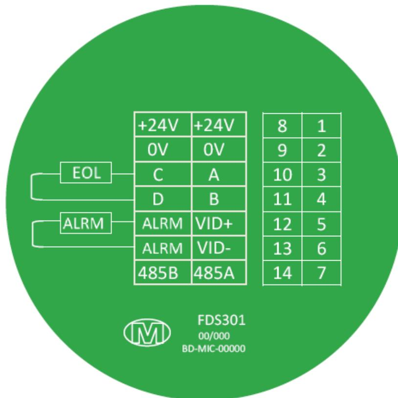
The detector has two types of alarm output available simultaneously
