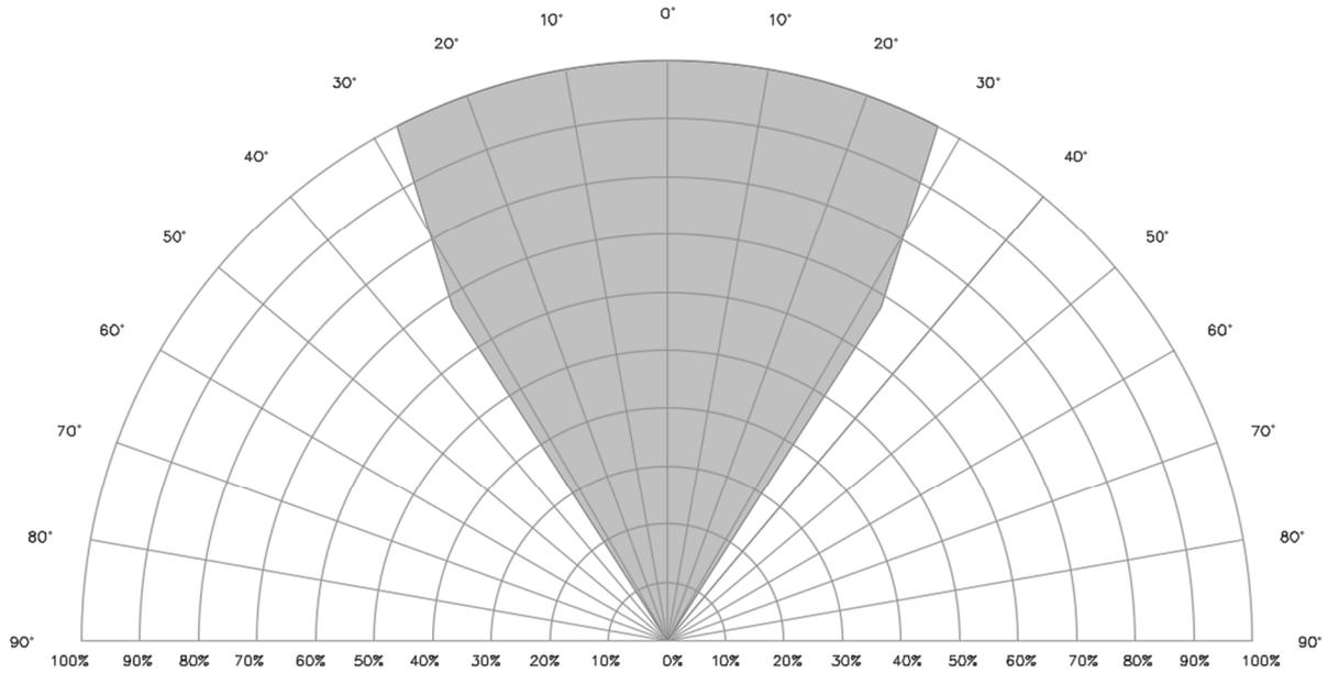
Vertical field of view to a 0.1 metre<sup>2</sup> N-heptane pan fire with an alarm response time of less than 30 seconds 100%=44 metres
