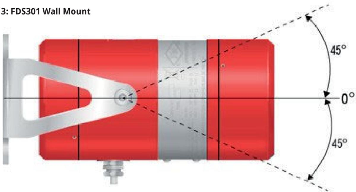
Firm, vibration free mountings are essential for trouble free operation of optical systems and the detector should be fixed to a rigid mounting. When mounting on a wall in this orientation allow for the cable gland and cable as this may restrict the downward rotation of the detector.
