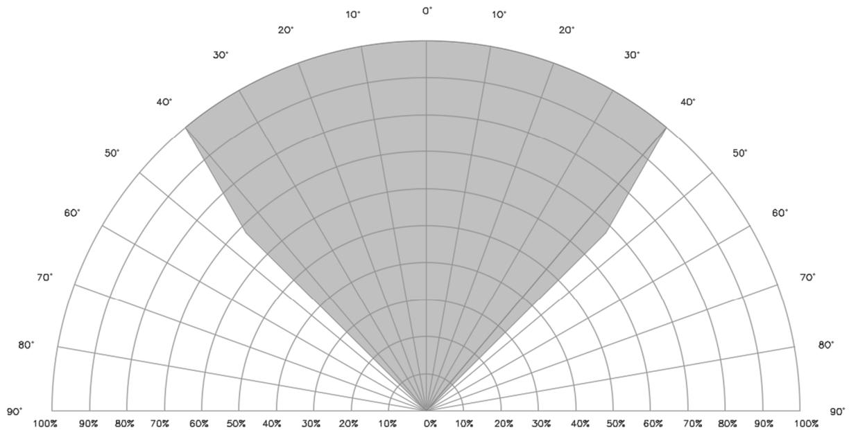
Horizontal field of view to a 0.1 metre<sup>2</sup> N-heptane pan fire with an alarm response time of less than 30 seconds 100%=44 metres
