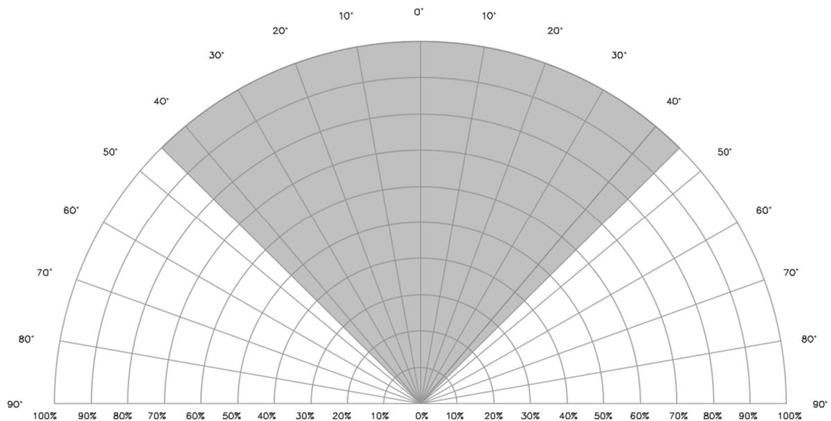
Vertical field of view to a 0.1 metre<sup>2</sup> N-heptane pan fire with an alarm response time of less than 10 seconds 100%=44 metres
